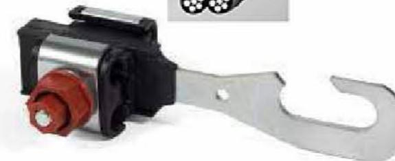
Anchoring Clamp 4x16-35mm<sup>2</sup> PAC 80 is used in power networks conducted by LV ABC of cross-section from 4x16mm<sup>2</sup> to 4x35mm<sup>2</sup>. Tightening is achieved via shear head nut of maximum tightening torque of 18 Nm. Minimum breaking force is 7,5 kN.
