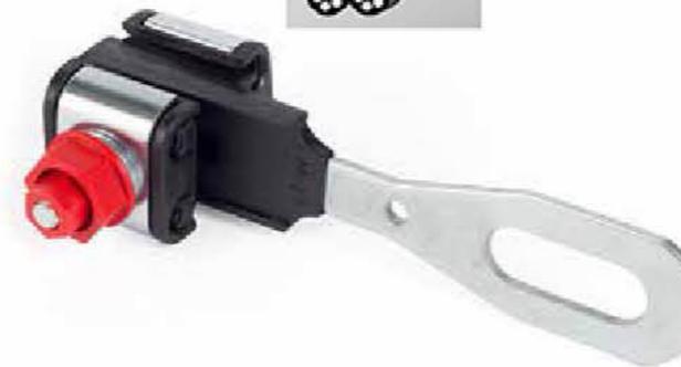
Anchoring Clamp 4x16-35mm<sup>2</sup> PA 80 is used in power networks conducted by LV ABC of cross-section from 4x16mm<sup>2</sup> to 4x35mm<sup>2</sup>. Tightening is achieved via shear head nut of maximum tightening torque of 18 Nm. Minimum breaking force is 7,5 kN.
